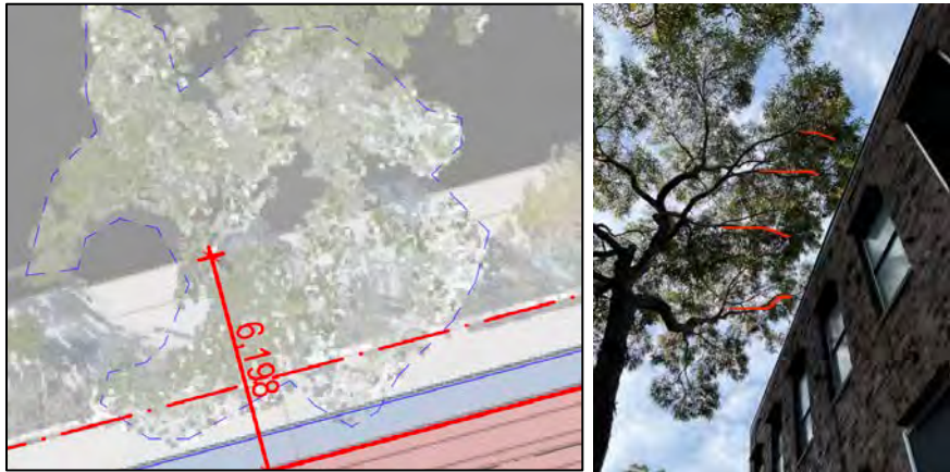
Figures 76 & 77: The Tree canopy impact of the proposed building in Pink and 1m wide scaffold in Blue. (Left) (Source: Tree Canopy Modelling by Plus Architects dated 1/08/2023) and The proposed pruning requirements to accommodate the proposed building façade next to Tree 14. (Source: Austin 2 nd November 2023).
