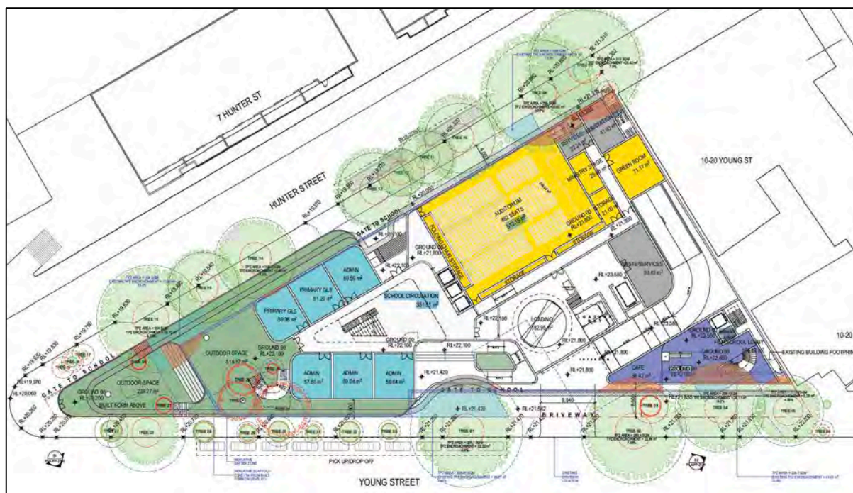
Figure 33: The floor plan depicting the existing building in the blue hatched line with the proposed building TPZ encroachments shown in pink, batter in blue and scaffold from level 1 and above shown in hatch (Source: General Floor Plan, by Plus Architects, drawing number PLA-PP -1000 dated 21/12/2024). See appendix for larger plans.
